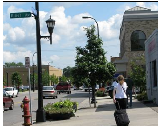
The street lighting on this section of Franklin Avenue serves both pedestrian and vehicular needs through a combination of low-level ornamental lighting and high-level shoebox style lighting.
