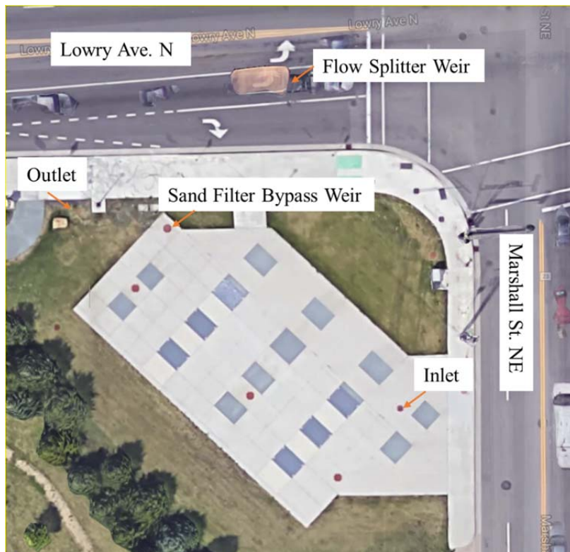
Figure 14-2. Aerial photo of The Lowry Sand Filter with the flow splitter weir, inlet, sand filter bypass weir, and outlet.
