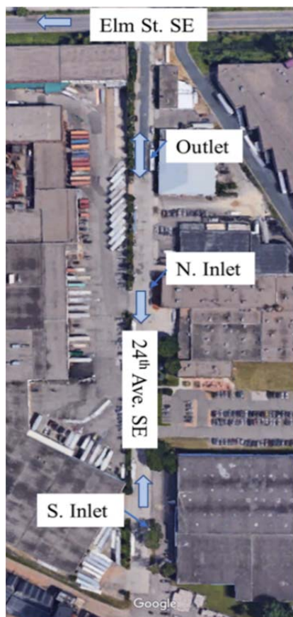
Figure 14-9. Aerial photo of 24 th & Elm Infiltration Chamber. Blue arrows show the direction of flow.
