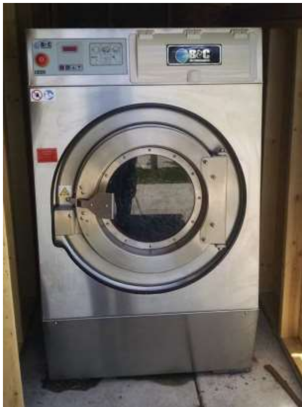
Figure 14-35. The industrial washing machine used to rinse filters.
