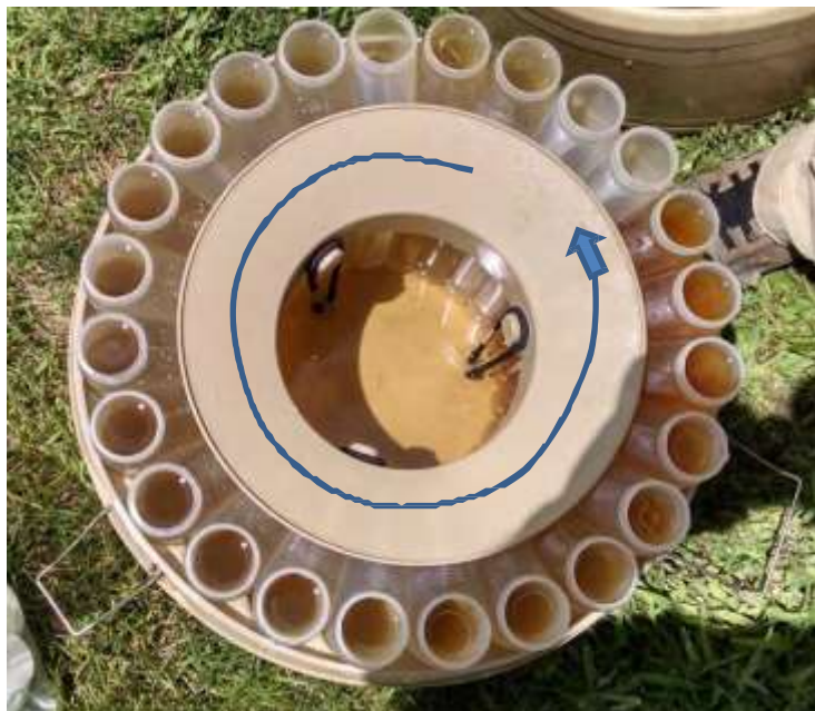
Figure 14-11. The 2015 37 th & Morgan Outlet samples. Starting at 1 o'clock and moving counter clockwise samples progress through the storm.
