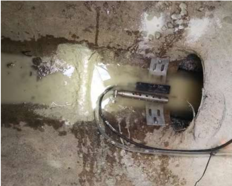
Figure 14-32. Webber Pond North Inlet 12 inch RCP pipe with AV probe and intake strainer. In 2016, a 1-inch berm was built downstream at both Inlet sites. The cement berm was built to pool water and help collect samples at low flows.
