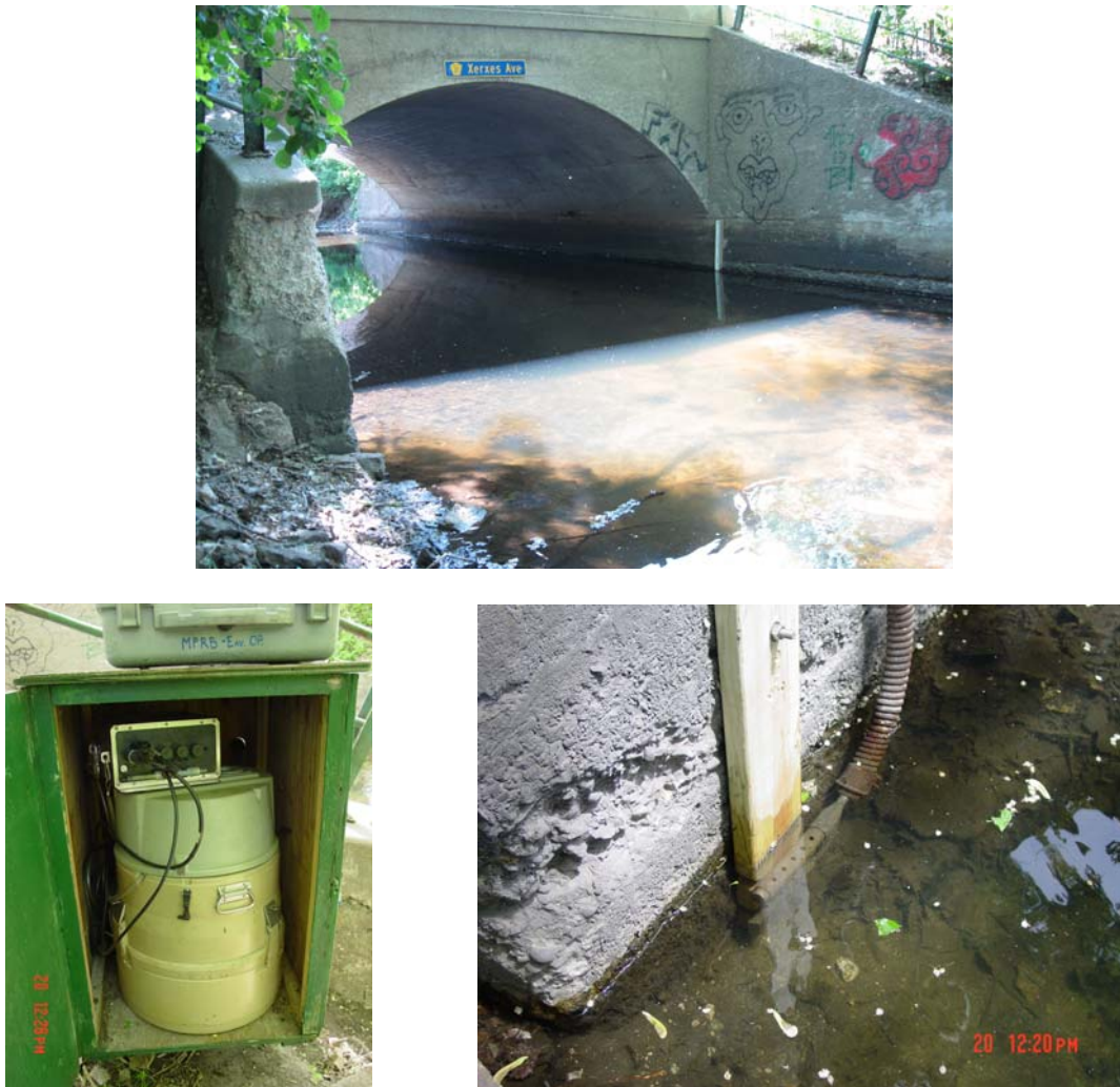
Figure 26-2. Top: Xerxes monitoring station location at Minnehaha Creek. The staff gauge as a vertical white line in the middle right. Left: Doghouse installation with sampler and datalogger. Right: Close up of intake strainer and level probe anchored to the northwest bridge abutment.
