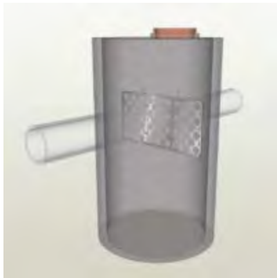
Figure 14-2. Drawing of a SAFL baffle in a sump. Baffle in the diagram is perpendicular to flow, unlike the baffles in the study site.
