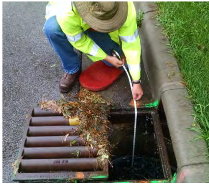
Figure 14-5. Measuring a tapedown from a fixed point to the catch basin.
