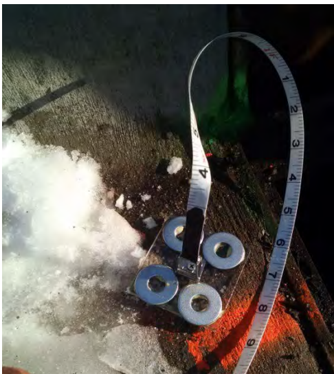
Figure 14-4. Showing tapedown foot construction.
