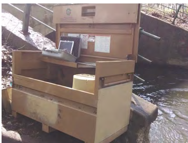
Figure 26-2. Top: Xerxes monitoring station location at Minnehaha Creek looking downstream. The staff gauge is a vertical white line in the middle right. Left: Knaack box installation with sampler and datalogger. Right: Close up of intake strainer and level probe anchored to the northwest bridge abutment.
