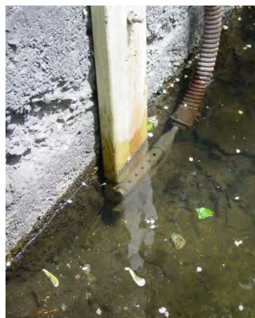
Figure 26-2. Top: Xerxes monitoring station location at Minnehaha Creek looking downstream. The staff gauge is a vertical white line in the middle right. Left: Knaack box installation with sampler and datalogger. Right: Close up of intake strainer and level probe anchored to the northwest bridge abutment.
