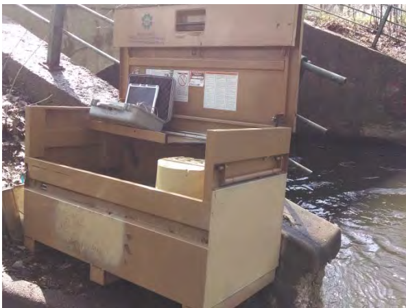
Figure 26-2. Top: Xerxes monitoring station location at Minnehaha Creek. The staff gauge is a vertical white line in the middle right. Left: Knaack installation with sampler and datalogger. Right: Close up of intake strainer and level probe anchored to the northwest bridge abutment.
