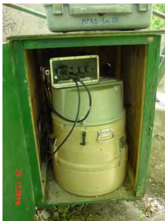
Figure 26-3. Left: Doghouse installation with sampler and datalogger. Right: Close up of intake strainer and level probe anchored to the northwest bridge abutment.
