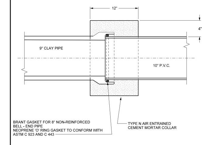
NOTES: P.V.C. = POLYVINYL CHLORIDE PIPE C.P. = STANDARD STRENGTH CLAY PIPE MINNEAPOLIS CUSTOM MNDOT SPEC. REF. 3245, 3251 NOT TO SCALE
