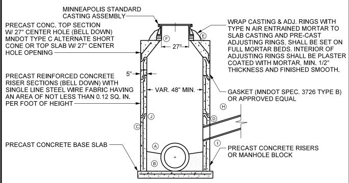
FOLLOW MNDOT 2451.3-C - FOUNDATION PREPARATION AND COMPACTION REQUIREMENTS OF MNDOT 2105.3 F1 - SPECIFIED DENSITY METHOD (100% COMPACTION REQUIREMENTS OF STANDARD PROCTOR)
