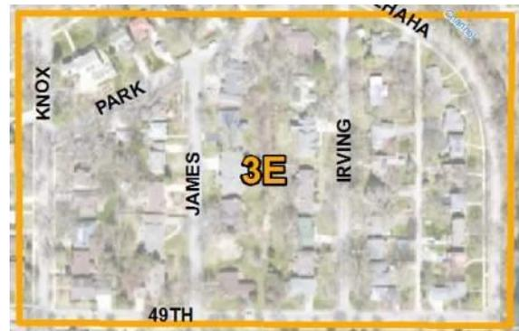
The improvements achieved in Subarea D also allow additional stormwater conveyance out of Subarea E. Any backyard drain connections to further reduce ponding extents would require City storm sewer improvements along 49<sup>th</sup> Street that are not proposed as part of this study. Should residents choose to tie in to the City system, further analysis of the 49<sup>th</sup> St system will be required.
