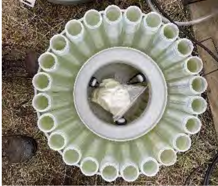
Figure 6. Photo of ISCO 3700 autosampler base with flow-weighted composite samples inside.
