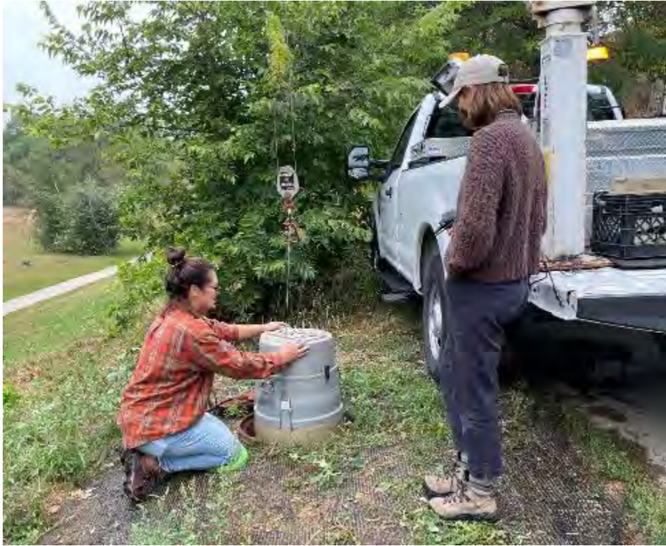
MPRB staff collecting stormwater composite samples at a Powderhorn monitoring site, summer of 2023
