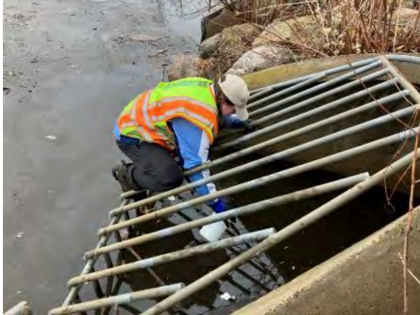
Figure 5. Staff collecting a winter snowmelt grab sample from the Camden Inlet N NW pipe. Snowmelt samples occasionally need to be collected at the pipe outfalls rather than the access manholes due to thick snow/ice coverage and for staff safety.
