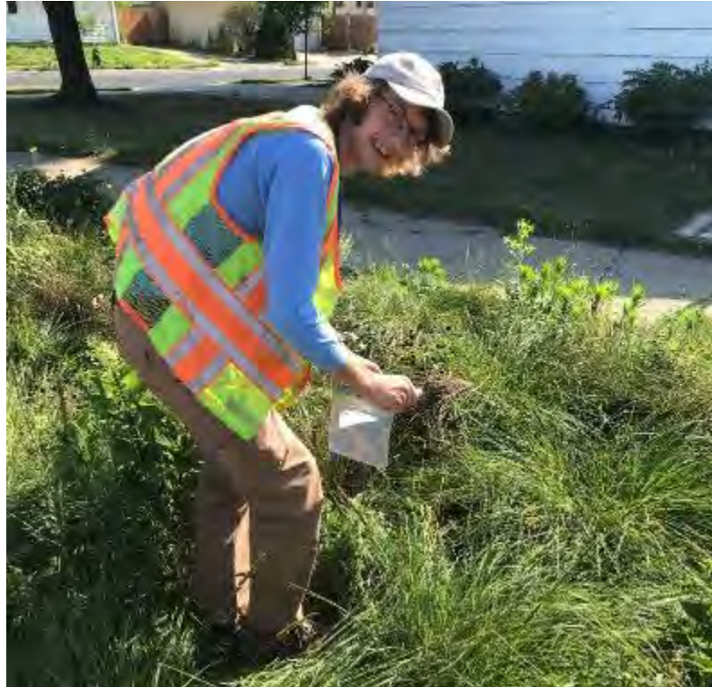
Figure 3. A soil sub-sample being collected by MPRB staff at the Hoyer A GSI site.
