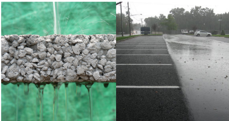
Left: Pervious concrete. Right: Porous asphalt compared to traditional asphalt.
