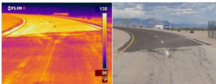
A test road at the Lawrence Berkeley National Lab is shown with partial light-colored pavement and partial dark or "normal" pavement. The image on the left shows that the lighter pavement is about 17°C (30°F) cooler than the darker pavement.
