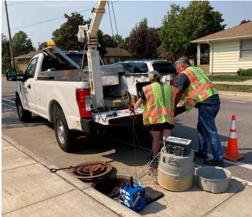
Figure 10. MPRB staff reprogramming the sampler at Camden S NW.
