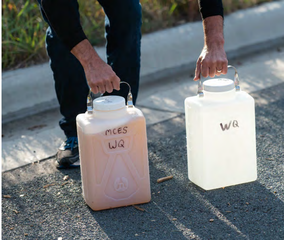
Figure 6. Samples of the clear inlet water, right, and colored underdrain outlet water, left, during the Hoyer GSI flood/hydrant test on October 4 th , 2022.
