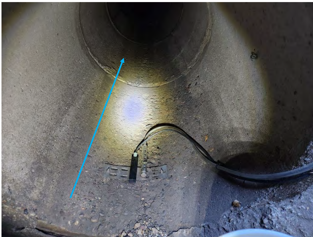
Figure 5. Photo of the AV probe and intake strainer at Powderhorn Inlet SE in October. The equipment is attached to a stainless-steel plate that is bolted into the pipe. The blue arrow indicates direction of water flow.
