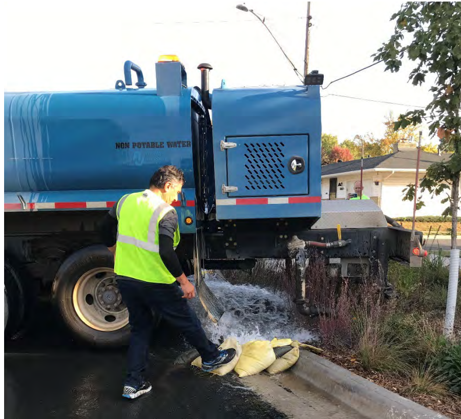
Figure 5. A flood test on 10/4/2022 at Hoyer A. Sandbags were used to direct flow into the grate.
