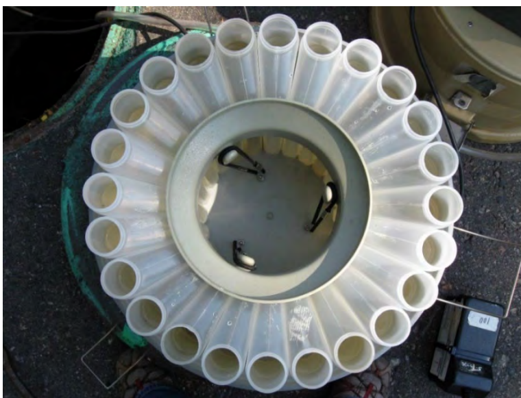
Figure 6. Photo of ISCO 3700 autosampler with flow-weighted composite samples inside.
