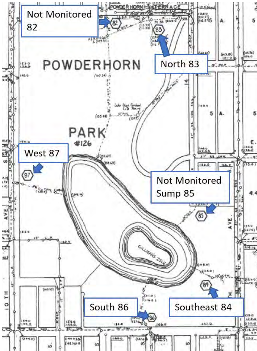
Figure 24-3. Storm sewer map of CDS grit chambers 82-87 surrounding Powderhorn Park.
