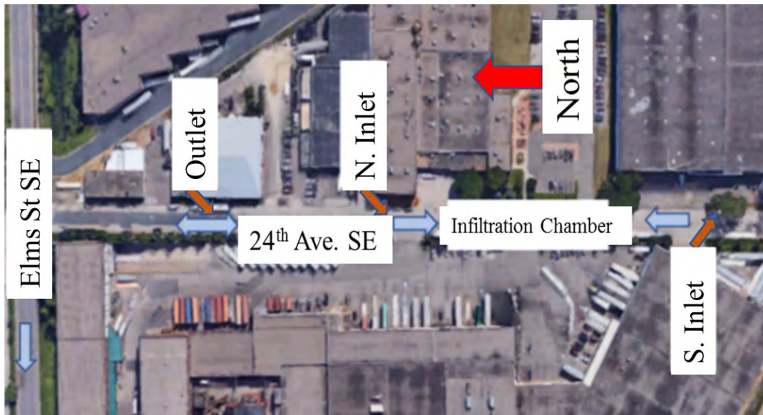
Figure 23-2. Aerial photo of 24 th & Elm Infiltration Chamber and its inlets and outlet. Blue arrows show the direction of flow. Only the inlets were monitored for FOG.
