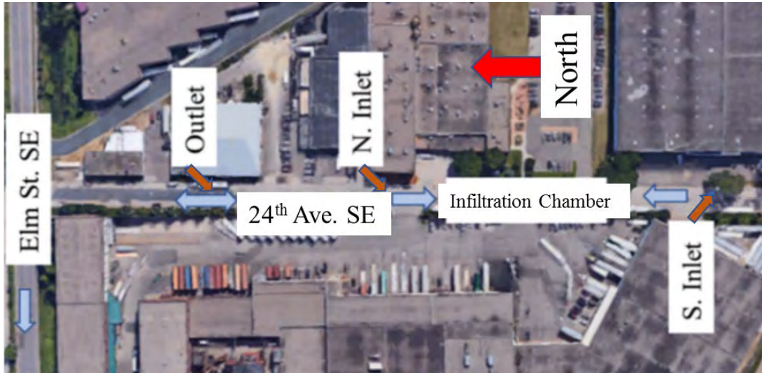
Figure 26-1. Aerial photo of 24 th & Elm Infiltration Chamber and its inlets and outlet. Blue arrows show the direction of flow.
