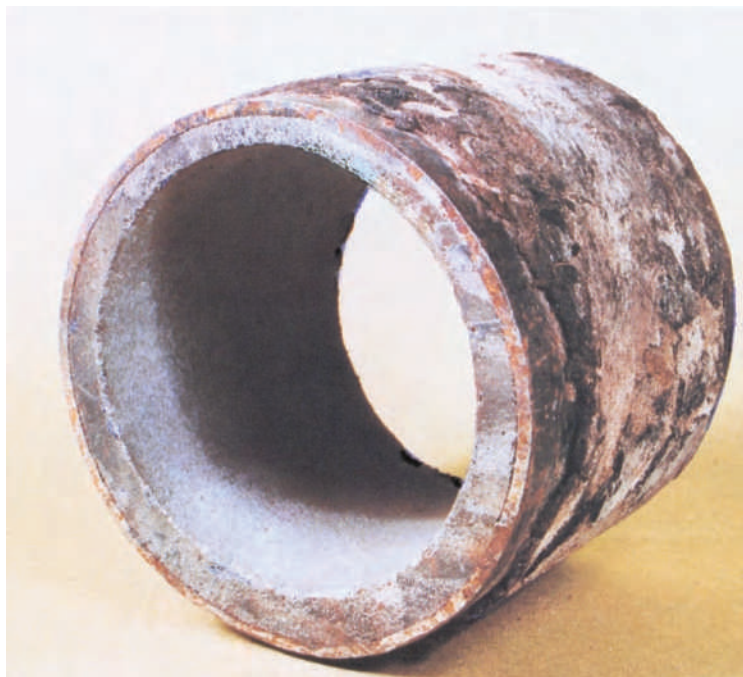
Pipe cleaned & lined
