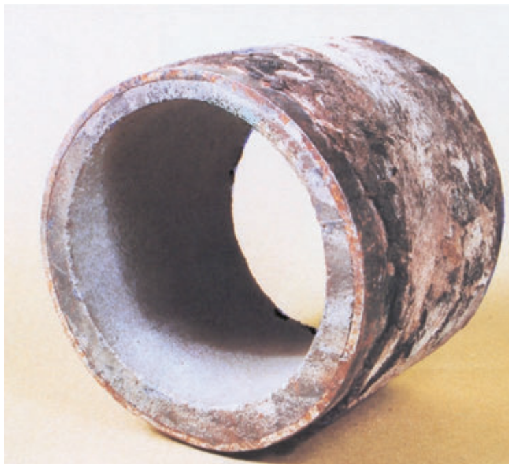
Pipe cleaned & lined
