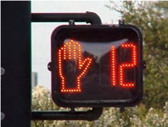
Pedestrian Signal with Count-down Timer
