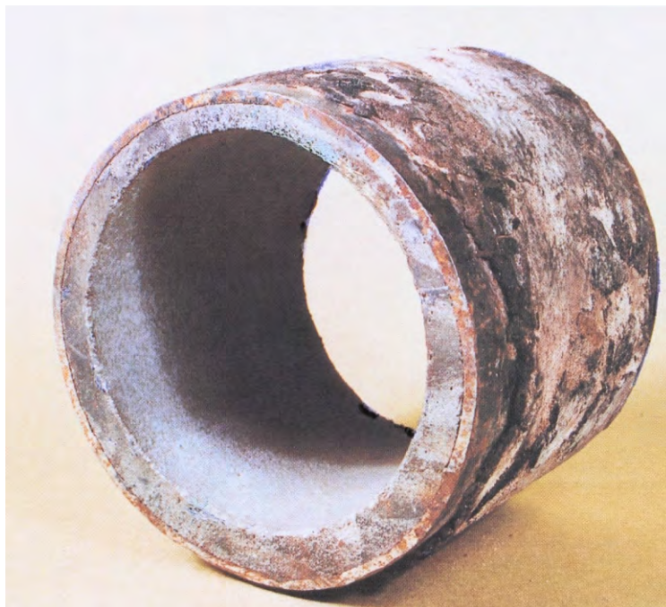
Pipe cleaned & lined
