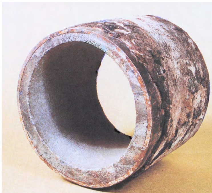
Pipe cleaned & lined
