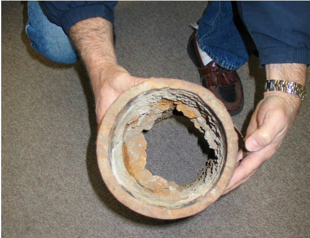
Water pipe before cleaning
