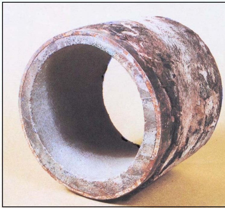
Pipe cleaned & lined
