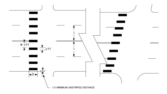
\* MARKED AREAS TO BE CENTERED ON CENTERLINE AND LANE LINES. SPACE UNIFORMLY TO AVOID WHEEL PATH.
