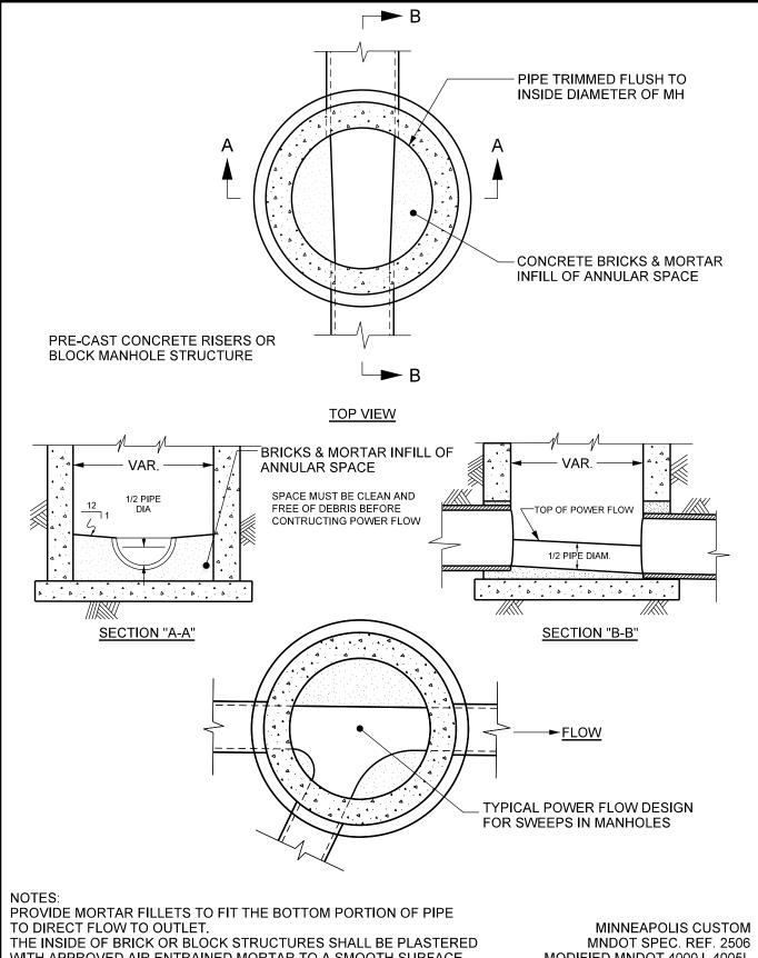
WITH APPROVED AIR ENTRAINED MORTAR TO A SMOOTH SURFACE. POWER FLOW STANDARDS APPLY TO ALL MANHOLE STRUCTURES.
