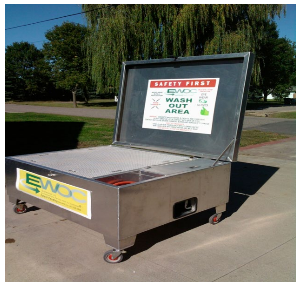
Self-contained washout facility
