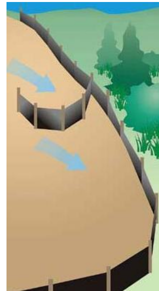
"J-hooked" silt fencing
