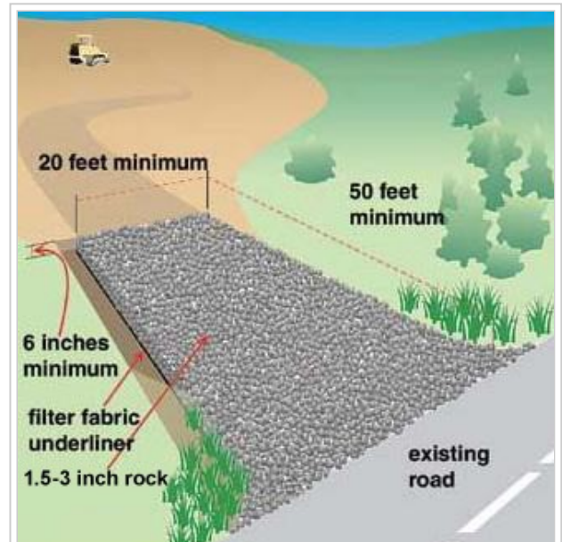
Vehicle tracking rock pad at site entrance/exit rock. Source: Created by Tetra Tech for US EPA and State of Kentucky.
