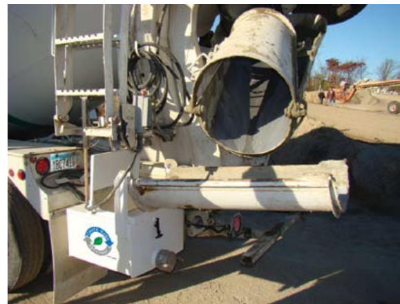
Recover and recycle wash water back into the truck
